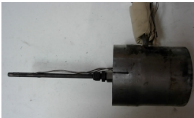
Figure 2: Exhaust probe, mount, and sample line
