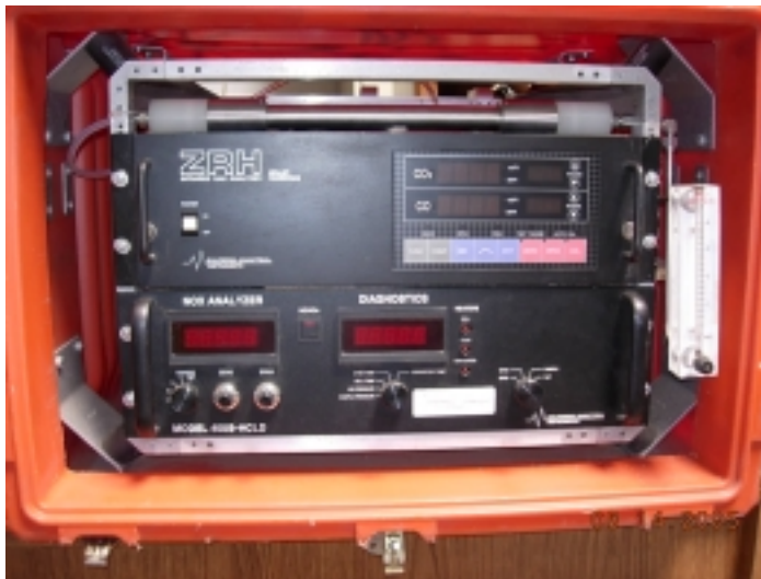
Figure 3: RAVEM gas analyzer system in shock-mounted case
