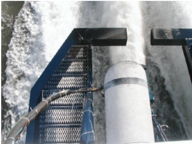
Figure 2: Sample line to the port main engine exhaust, high speed cruise conditions, Mare Island
