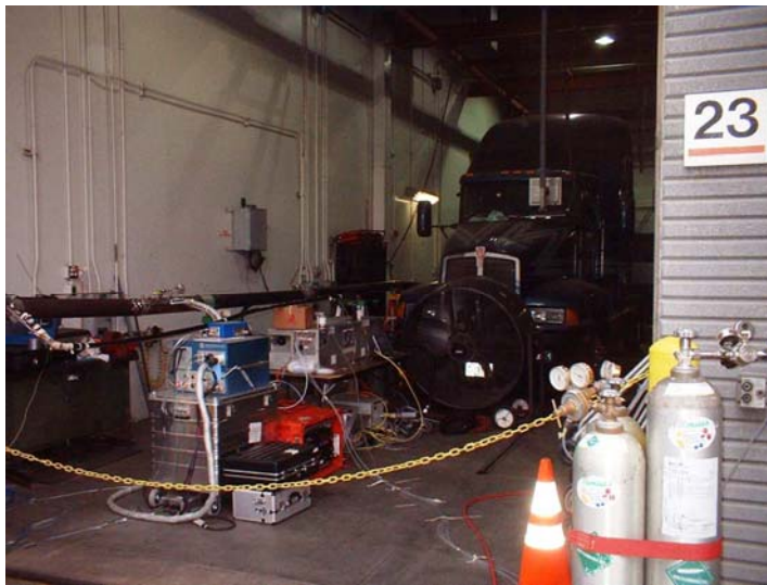
Figure 2: Test truck and extended exhaust pipe with PEMS systems installed
